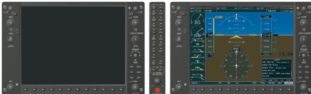
Figure 2.7.2 G1000 Reversionary Mode (Failed PFD)
